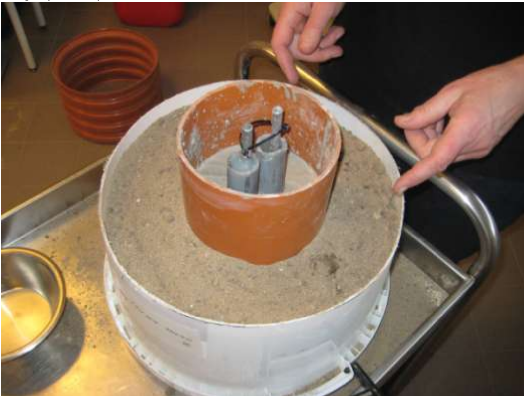
Figure 2.2: One of the lab “boreholes” during construction. The orange PVC pipe represents the casing and is removed before the test is carried out.
