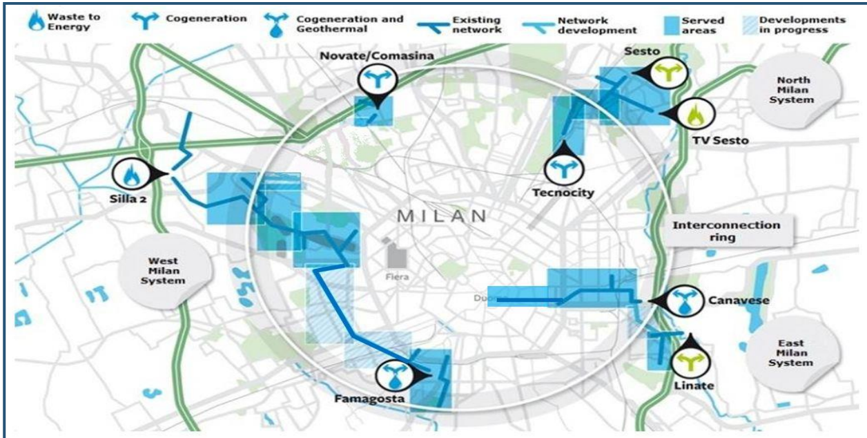
Figure 4. Interconnection status and plans for the different networks in Milan. [6]
