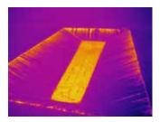
A thermal image shows status of the water filling during the winter of 2021. An irrigation system has been developed to protect the liner during filling.
