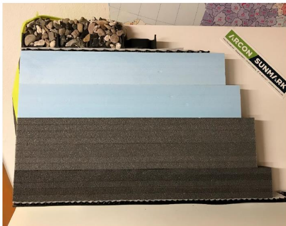
Figure 11: Cross-section of mock-up model of Aalborg CSP's lid construction.
