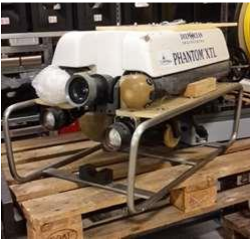
Figure 25: Phantom XTL underwater drone
