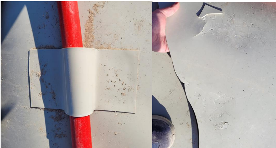
Figure 18: PP strap attached to PP liner and crack in PP liner.
