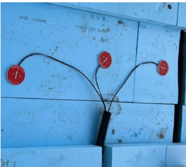
Figure 24: Location of Hukseflux heat flux meters in the insulation (top view).
